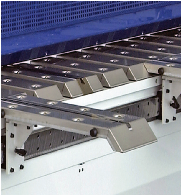
Linear guide, at the front for movable table support arms and table with ball rollers
